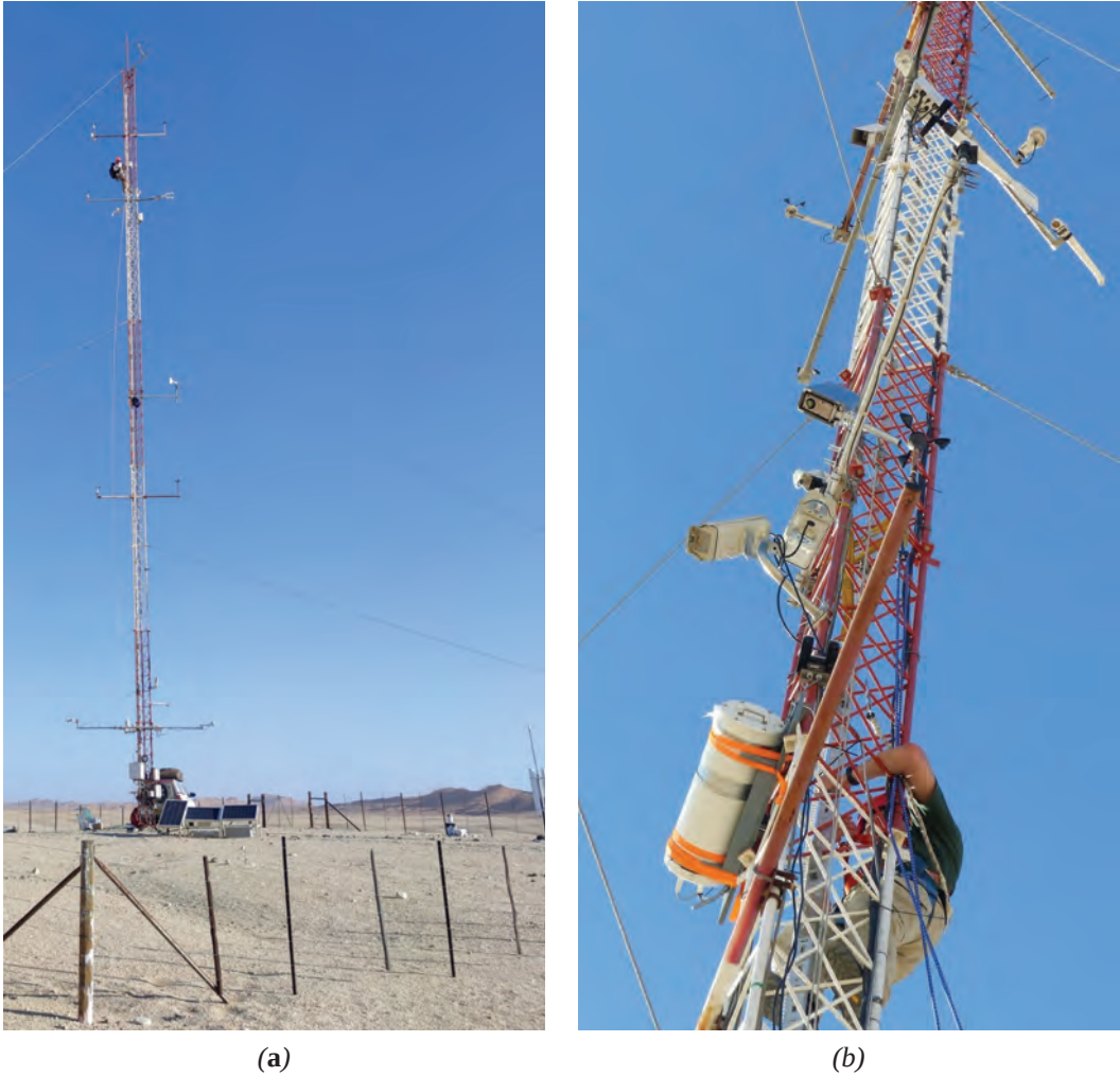
Figure 1: Land Surface Temperature (LST) at validation station Gobabeb. (a) wind tower (b) installation of different radiometers during the 2017 ESA FRM4STS field inter-comparison experiment
