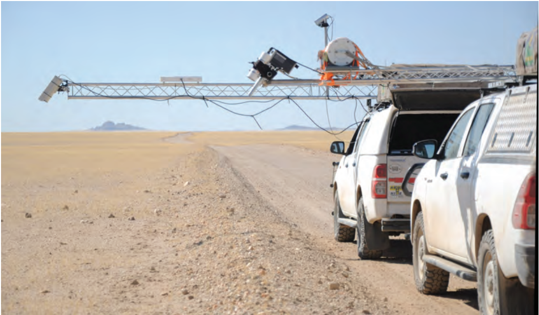
Figure 3: Characterizing LST homogeneity of the gravel plains between Gobabeb and Mirabib. The five TIR radiometers participating in the ESA FRM4STS field inter-comparison experiment (Götsche et al. 2018) provided spatially resolved in situ LST along the driven track.
