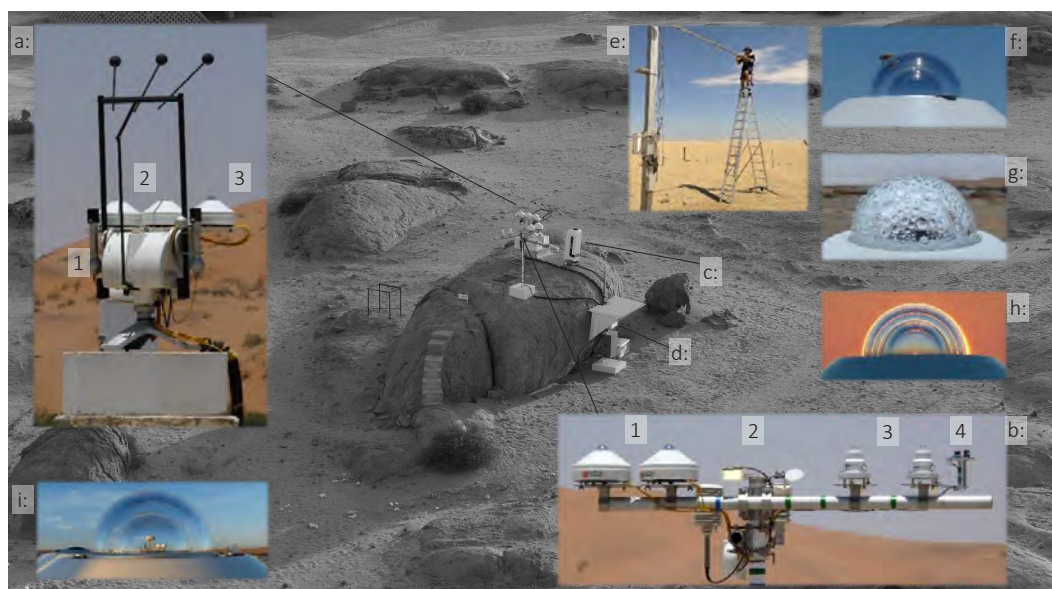
Figure 3: Grey background: View to the BSRN station on the rock with the downwelling flux measurements. a: Tracker positioning two pyrhemometers (1) and shadow balls for two pyrgeometers (2) and one pyranometer (3) with sun close to zenith. b: Boom holding two pyranometers (1), meteorological instruments (2), one UV-B pyranometer and one UV-A pyranometer (3) and two PAR sensors (4). c: Ceilometer. d: Data acquisition and power supply. e: upwelling flux measurements. f: a fly casting a shadow for qualifying uncertainty. g: fog deposition on a dome. h: sunset in a pyranometer. i: Gobabeb water tower seen through the dome of the pyranometer for diffuse radiation.
